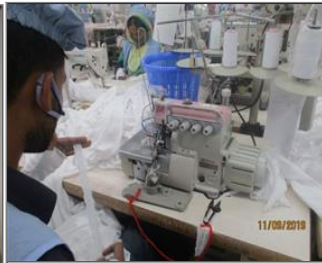
External photo(s) of the production unit(s) NC 7.17 Eye guards of overlock sewing machines in the sewing section were not proper place.JPG
