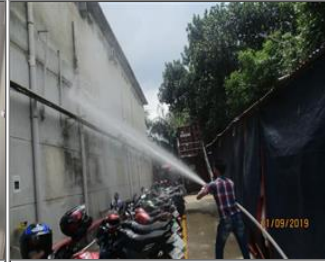
External photo(s) of the production unit(s) Fire hose test.JPG
