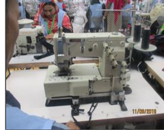
External photo(s) of the production unit(s) NC 7.17 Three needle sewing machines in the sewing section did not have needle guard.JPG
